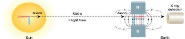
**X-files.** CAST "telescope" hopes to detect hypothesized particles from the sun by counting the x-rays they should produce on passing through an intense magnetic field.
